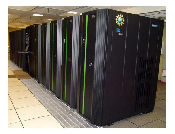
IBM Power 575: 128 nodes, 32 CPUs per node Each CPU is 4.7GHz, 4096 CPUs in total Weight is 33,000 lbs. not counting the circulating water cooling equipment.
